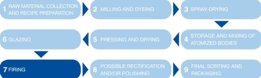
Inside the kilns the tiles move on rollers made of refractory material. The firing of the tile is made up of many sub-phases, depending on the different parts of the kiln itself.
