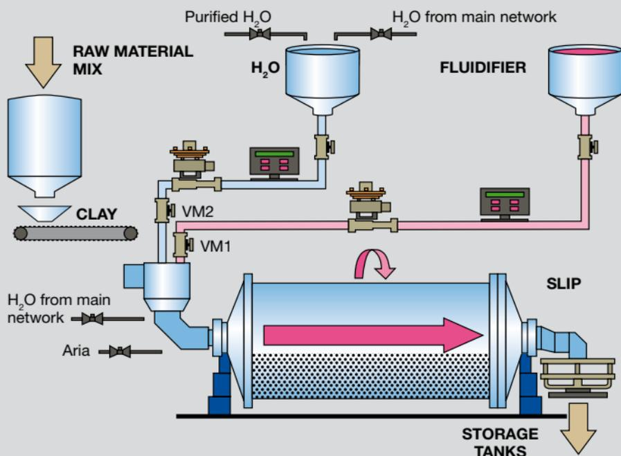
Chambers inside the continuous mill, which, as the mill itself, are separated by holed grids covered with rubber, contain milling bodies of decreasing dimensions and featuring a suitable size for the performance of the milling and refining. As the mixture moves on from the milling chamber inlet towards its outlet, the passage of the mixture from one chamber to the other takes place only at the moment it has reached a sufficiently “fine” granulometric size.
