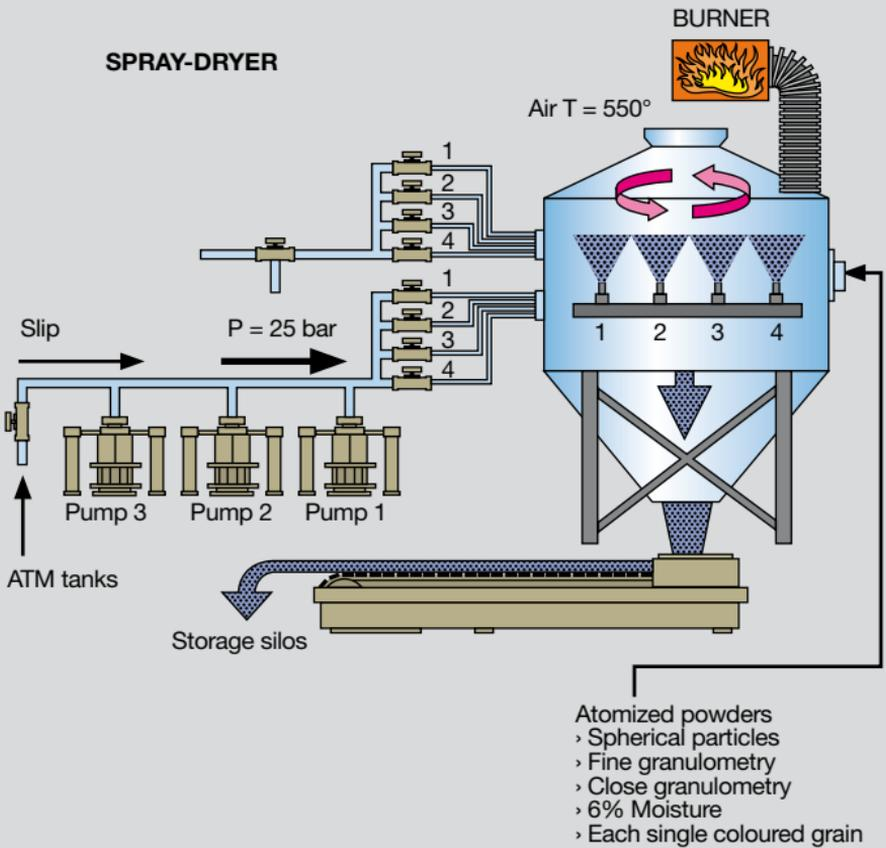
The slip contained in the tanks is collected via pumps then sent to the spray-dryer.
