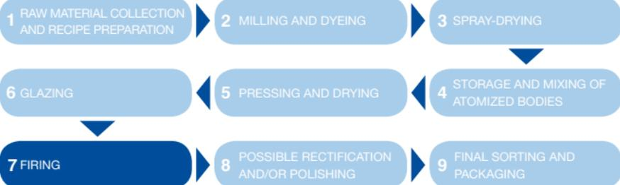
But why is a storage chamber needed both before and after the kiln? The productive capacity of any ceramic company much depends on the firing phase; therefore, it is essential for the kiln to be constantly full. Hence there are two storage phases at Italon, pre and post firing, in order to avoid that any unforeseen interruption in the tiles flow (from machineries upstream and downstream of the kiln), may cause slowdowns in production.
