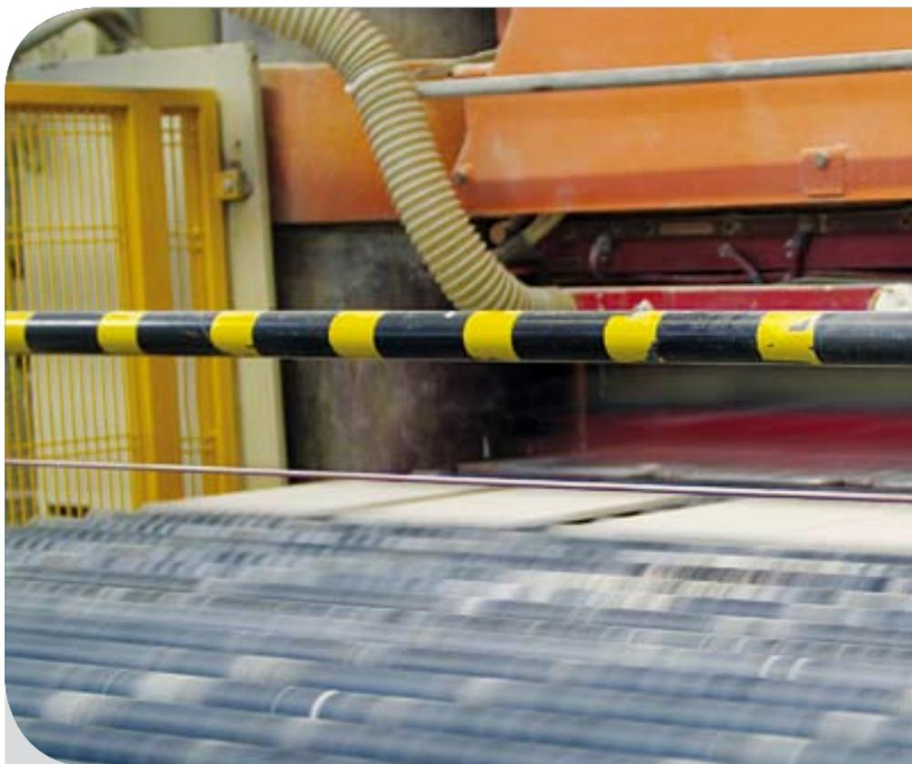
At this stage, the newly formed tile is not yet ready to be fired, as its moisture content is still too high. Therefore, it is placed on the device located below the press: the DRYER, whose purpose is that of bringing the moisture content of the tile to a level close to zero. At the end of the drying process, the tile reaches the production line at a temperature of around 80-100°C, the temperature needed for the tile to undergo further processing.
