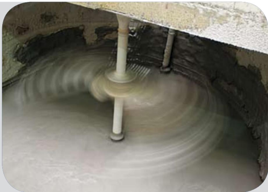
Each mill is provided with adjoining cavities, each of them containing a set amount of milling bodies, that, through rotation, fall one over the other, thus grinding and chopping the mixture.
