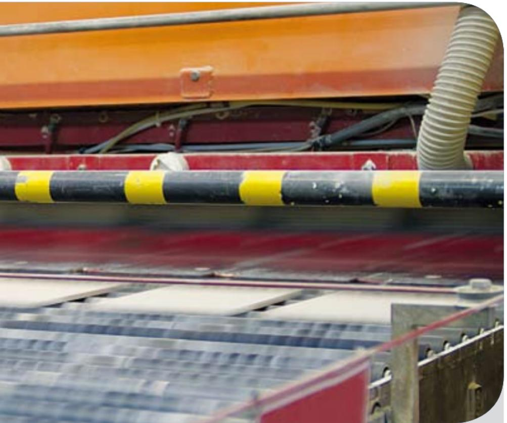
The dryers are eco-friendly devices as they produce heating power through the recovery of the heat produced by the kiln, thus allowing for considerable energy saving.
